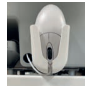
Mouse holder with a slot for the USB cable of a medical mouse
